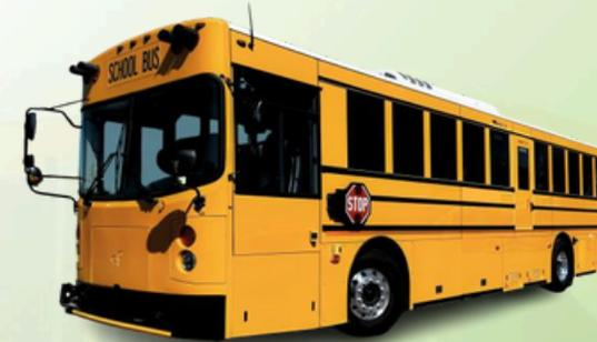
The BEAST is a unified structure that features a seamlessly integrated aluminum body on a high strength steel Truss (bus) chassis. Its complete flat floor design allows for tracking with no obstacles, and the high floors keep students out of the crash zone.
