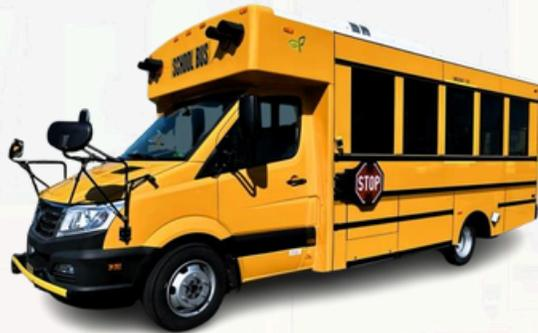
The award-winning Nano BEAST features a seamlessly integrated aluminum body. It is built on the EV Star Cab & Chassis which is the same foundation as the EV Star Passenger Van that passed the FTA Altoona Bus testing program with the second highest score of 92.2.
